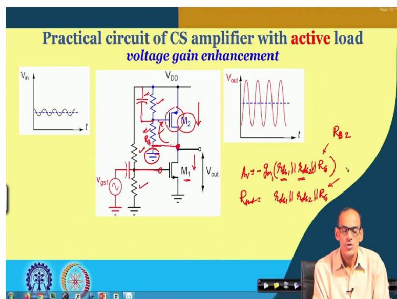
This is what it is shown here. I will not be going in detail, but just to say that we do have say one resistor here. We do have another resistor here to define the gate voltage of transistor-1 and likewise we do have two more resistors here to define the gate voltage of transistor-2. And then we have to ensure that these two  $I_{DS}$  and  $I_{SD}$  they should be equal and both of the transistors should be in saturation region.
