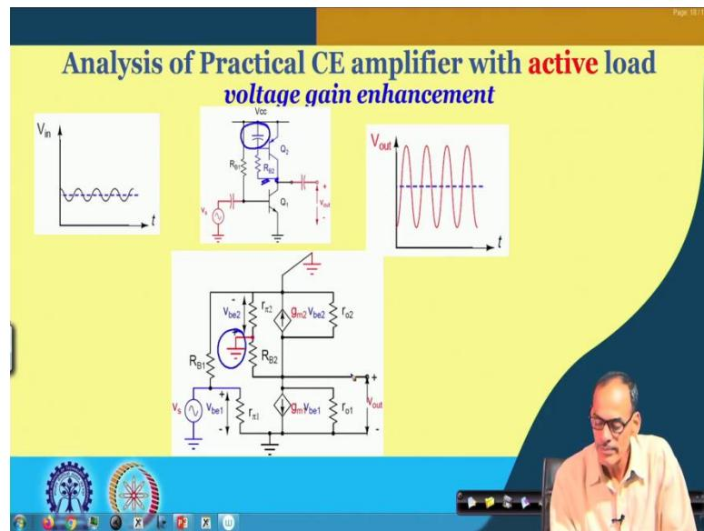
So, in summary of this modification what we like to say here it is. In this case by making the connection of this  $R_{B2}$  to the output node, we are making the operating point easily achievable. And then to avoid it is adverse effect on the gain namely the reduction of the gain we are putting this extra capacitor which is making the base node of transistor to ground and hence the corresponding gain it is remaining high. So, numerical value we will see it later.
