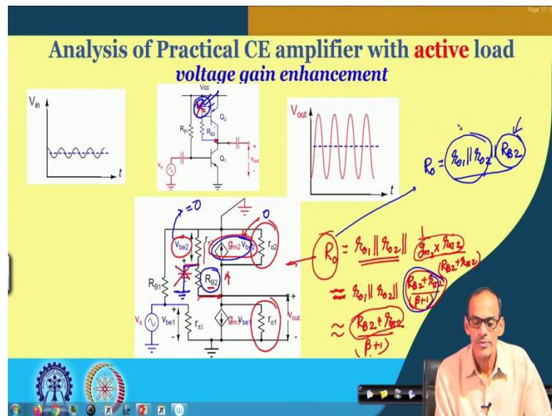
So, this is what the discussion here that if we connect this  $R_{B2}$  here; that means, this  $R_{B2}$  it is connected here it is not connected to ground. So, if we do not put this capacitor here then naturally then it will be providing one nonzero value of  $v_{be2}$  as a result this current it will be flowing as a non-zero entity. And there is a consequence in fact, looking into this circuit this active device it will provide additional conductance.
